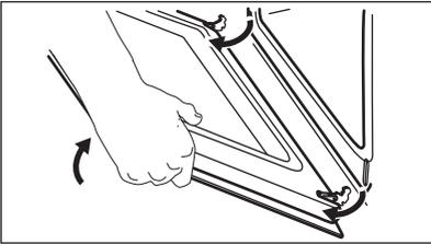
A line drawing showing a hand holding a door handle assembly. The hand is positioned at the top corner, and an arrow indicates the direction of force to push the hinge pin inward. The pin is shown being pushed into the handle's housing.            |
