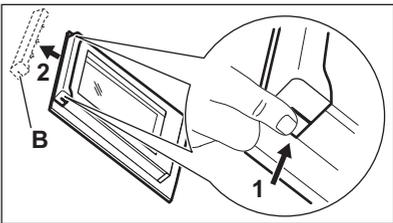
A line drawing showing a hand holding the top edge of a glass panel. An arrow labeled '1' points to the top edge. A label 'B' is placed near the panel. A circular inset shows a close-up of the hand holding the top edge of the panel.                |
